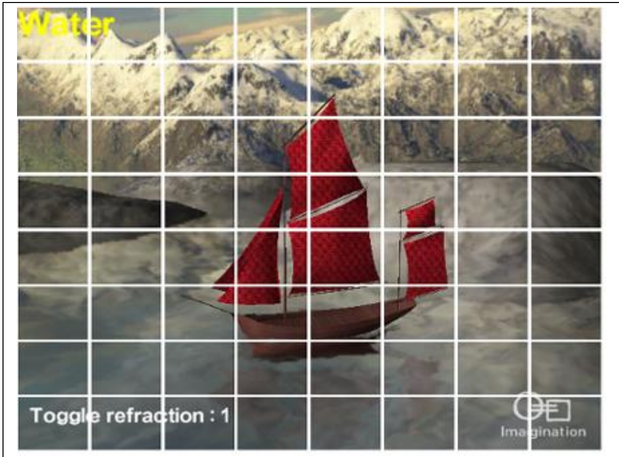
Figure 1 - Tile subdivision used to render a frame
